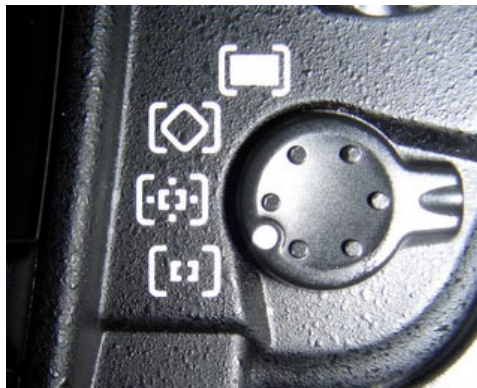
The Autofocus mode selector switch is on the back of the D2 series cameras
