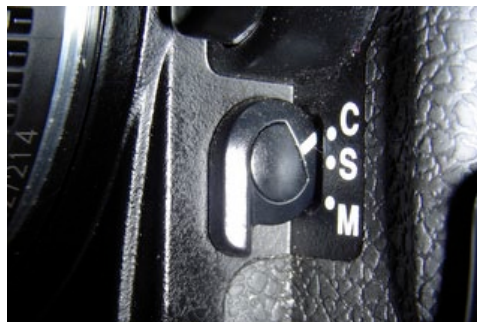
The servo mode selector switch is on the front of the camera, underneath the lens release button.
